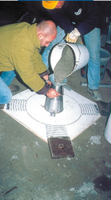
Slump flow tests on concrete manufactured with Stabilcem SCC
