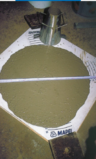
Measuring slump flow of concrete manufactured with Stabilcem SCC
