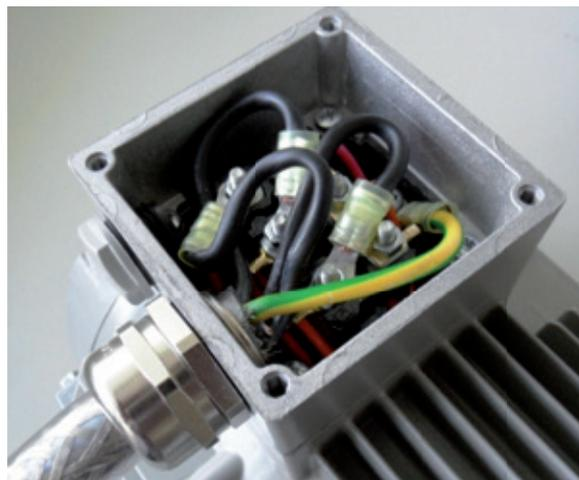
Wiring on the Motor Terminal Box
